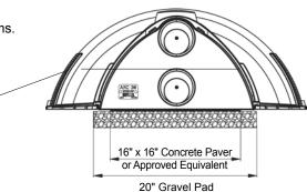
Use of 3" or Smaller PVC as Inlet Requires Use of Appropriate Hole Saw.
