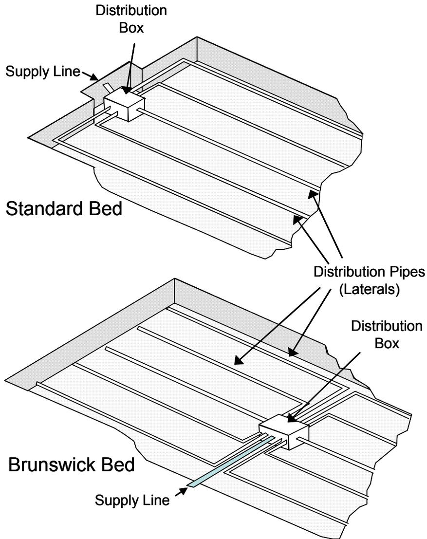
Figure 1. Schematic diagram of examples of the construction of standard and Brunswick bed/fill systems used in gravel systems in North Carolina.
