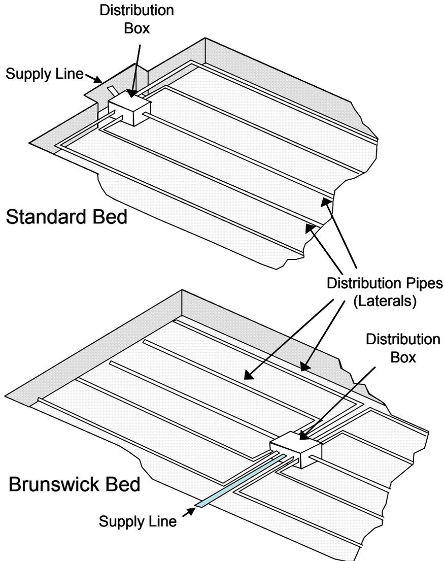
Figure 1. Schematic diagram of examples of the construction of standard and Brunswick bed systems used in North Carolina.
