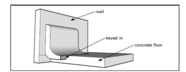
Example of quarry tile cove base integral to concrete floor.
