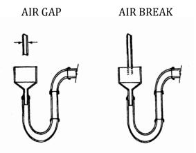
A connection to a sewer line may be direct or indirect. A direct connection may not exist between the sewerage system and any drains originating from EQUIPMENT in which FOOD, portable EQUIPMENT, or UTENSILs are placed, except if otherwise required by law. When a WAREWASHING machine is located within 5 feet of a trapped floor drain, the dishwasher waste outlet may be connected directly on the inlet side of a properly vented floor drain.
